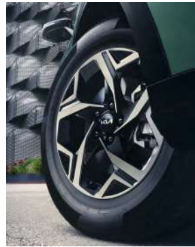
Alloy wheel 19", Type A. Bicolour, 7.5Jx19, suitable for 235/50 R19 tyres. 52910R2300PAC (GT-line exclusive)
